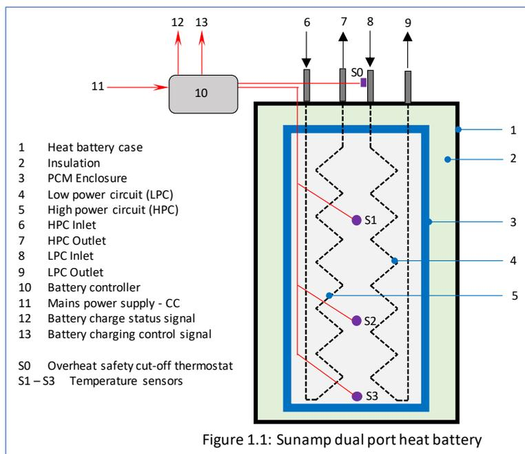
All Sunamp UniQ dual port heat batteries have two independent water circuits for transferring heat to and from the PCM heat storage material as shown *schematically* in Figure 1.1. Depending upon the application, the heat battery can be charged via a low power circuit (LPC) and discharged via a high-power circuit (HPC) or vice versa.
